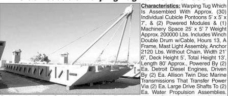
2120 Lbs. Without Chain, Width 21' 6". Deck Height 5'. Total Height 13'. Length 80' Approx., Powered By (2) Ea. Detroit Diesel Engines, Driven By (2) Ea. Allison Twin Disc Marine
