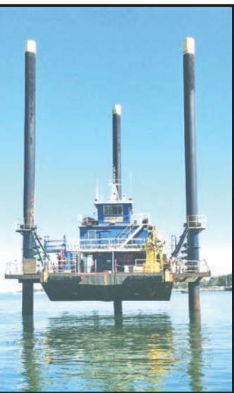
BAY SURVEYOR – CREW BOAT 45'x15'x3.5' CONVERTED TO ACCOMADATE DIVE CREWS AND SURVEY EQUIPMENT
