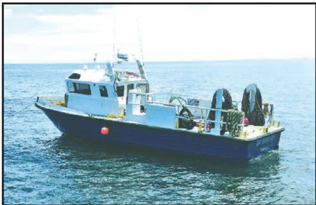
BAY SURVEYOR – CREW BOAT 45'x15'x3.5' CONVERTED TO ACCOMADATE DIVE CREWS AND SURVEY EQUIPMENT
