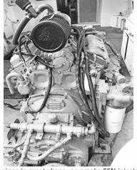
Engines in great shape, no smoke 55N injectors, keel cool R.T.O., Tonanco TM828S 1.96:1 transmissions. 7,000 hours, easy run at 1,500 RPMS or less. Gauge clusters with 60 foot wiring harness. Battery cables. Morse single lever controls with throttle / clutch cables 50 feet. Walker Air Seps. Remote oil change pump pan valve fitting. Ready to bolt up and run.
