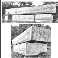
Two sectional barges 30' x 8' x 4' Boxed both ends. Connected size 30' x 16' x 4'. 14" sides and deck: 3/8" steel bottom.
