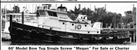
Charter Rates Available Upon Request - Sale Price: \$159,000. Main Engine: 12V71 Detroit Diesel 450hp @ 1800 rpm. Marine Transmission: Twin Disc MG 514 with 6:1 reduction. Shaft size: 4.5" steel. Aux Engine: 271 DD 20 kw genset 120/240 VAC 20 hrs, hydraulic steering. Capacities: Fuel oil 6,000 gallons in four (4) tanks. Potable water: 1500 gallons, Last DD, 2/14/17.
