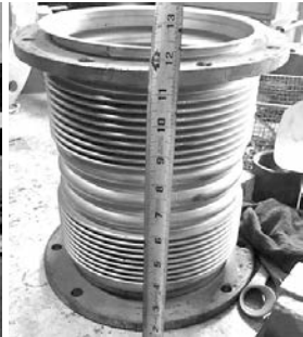
Exhaust Bellow For Cummins QSK Part #389756300 12" x 14" Double Wall Never Been Used
