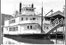
All Steel • Built 1965 Dubuque, Iowa Length 120' x 33' x 4' Draft (2) Detroit Diesel 8V-71 (1) Caterpillar 3304 - 100kW Generator Passenger Capacity 325 (2) Interior / (1) Exterior Levels
