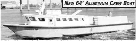
Built to ABS specs. Aluminum fast craft. #2 Northern Lights gens., 20KW. 4" stainless main shafts. 4" stainless rudder shafts. A/C 4 ton water to air heat pump. 15KW electric heat backup. Coast Guard approved 49 pax., 20 miles from coast. Powered by (2) Cummins QSK 19 800
