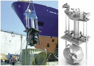
ZF Retractable Azimuth Tunnel Thruster Technology For R/V Roger Revelle
