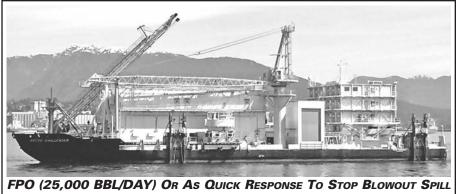
Ice Breaker Hull; ABS; Living Quarters 72 People (Certifiy for the Artic); (5) CAT Gensets; 4.5 MW Two Sparrow Cranes for 80 and 40 T; ROV; QXP25; 3000 M; Hydraulic Winch; Umbilical; LARS and \$250,000 Spare ROV Parts; Mooring Anchor; (8) Anchors (100 Tons Each); Offshore Well Intervention System. I Separate Crude Oil, Gas and Seawater 25,000 BBL/Day.
