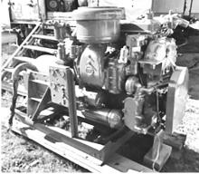
Naturally Aspirated 471 GM 60kW 1800 RPM Gen Set 1850 Hours • Hydraulic Shutdown
