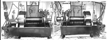
With air brakes and Hrydrostar 5 hydraulic motors. Drum capacity 285 fathoms of 1" wire (per winch).
