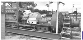
This is a 16" x 16" GIW Booster Pump with a CAT D398 Engine Booster is in work ready condition Booster has been serviced. blasted and painted Ready for inspection Weight: 40,000 lbs.
