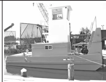
MODEL 2514 25'9" x 14'0" x 5'0" 600 H.P. Twin Engine
