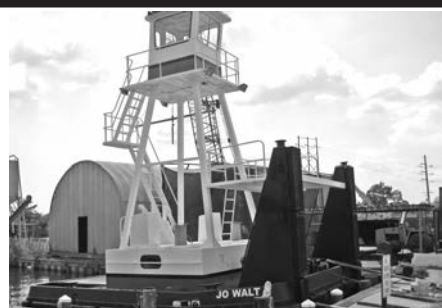
MODEL 2520 25'9" x 20'0" x 6'10" 750 H.P. Twin Engine
