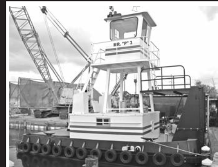
MODEL 2516 25'9" x 16'0" x 5'6" 650-750 H.P. Twin Engine
