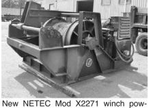
ered by 100 hp electric motor. Single drum with a spare drum. Drum A 1" wire rope 2,000 ft. Line pull final layer 10,000 lbs. Drum B ½" electromechanical cable 14,400 ft. with slip rings. Full specs and build drawings avail. Winch was built for scientific research.
