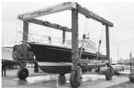
1988 35BFM - 70,000 lb. Capacity, 17' Inside Clear Width, 18' Inside Clear Height, Ford Gas Engine, Front & Rear Powered Slings. Loc. - Fall River MA
