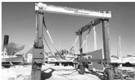
2000 35BFM - 77,000 lb. Capacity, 17' Inside Clear Width, 18' Inside Clear Height, Ford Gas Engine, Front & Rear Powered Sling.
