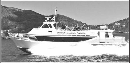
**Dream Speed** - Extremely comfortable mono hull 71ft SOLAS vessel that accomodates 149 Passengers plus crew. Two levels seats 98 in leather chairs with full AC and Flat Screens, and 54 on Sundeck. 2 Rest Rooms. Cruising at 28 knots fully loaded with luggage. US Coast Guard inspected and certified. If you are looking for a reliable ferry to supplement your fleet or start up a new service call:
